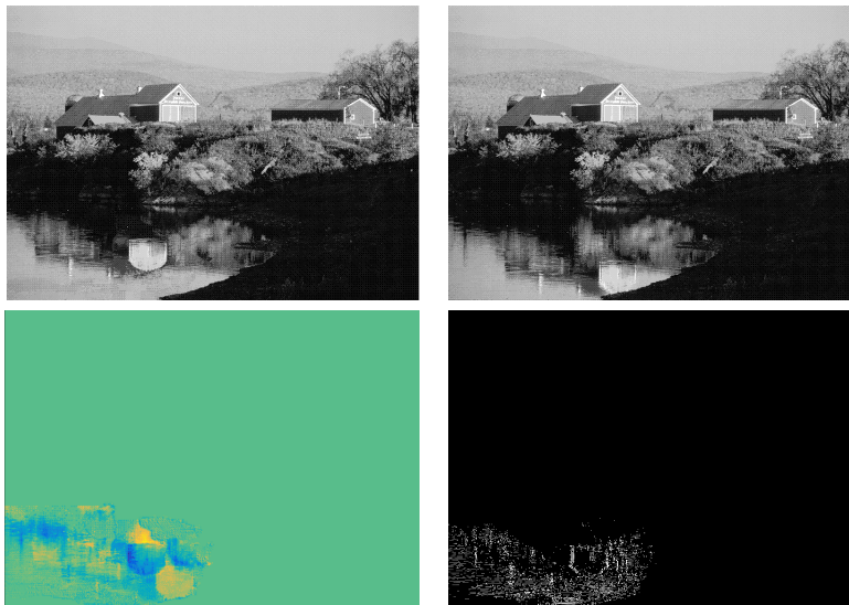
FIGURE 8. The two frames of the flickering sequence containing information (top), the difference between these two frames (down left), and the \vec{u}^{(2)} flow field resulting from the proposed approach (down right). As predicted in Section 3 and Appendix A the \vec{u}^{(1)} component is negligible, instead \vec{u}^{(2)} detects the change of intensity across the blank sheet.
